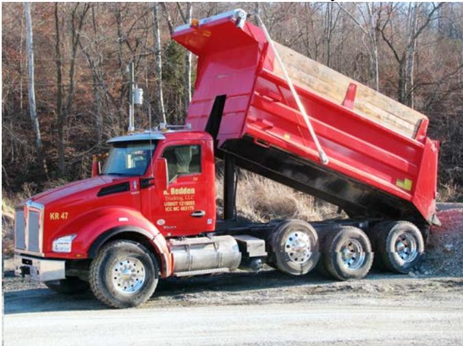
Redden also has a second T880 on order, with delivery expected soon. The T880 dump in operation is powered by the PACCAR MX-13 engine rated at 455-hp, and driven through a 10-speed transmission.
